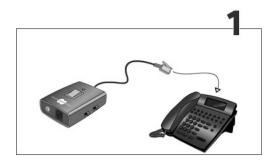
Take the headset cord out of the telephone and insert the pre-installed cord from the Busylight box into the telephone instead.
