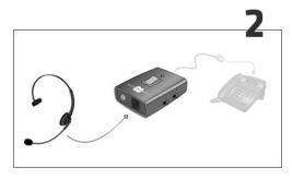
Insert the headset cord (that was in the telephone before) in the front of the Busylight box.
