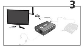
Insert the cord for the Busylight lamp into the Busylight box and mount the lamp on your screen (or another visible place) with the round tape. Avoid placing the lamp in direct sunlight.
